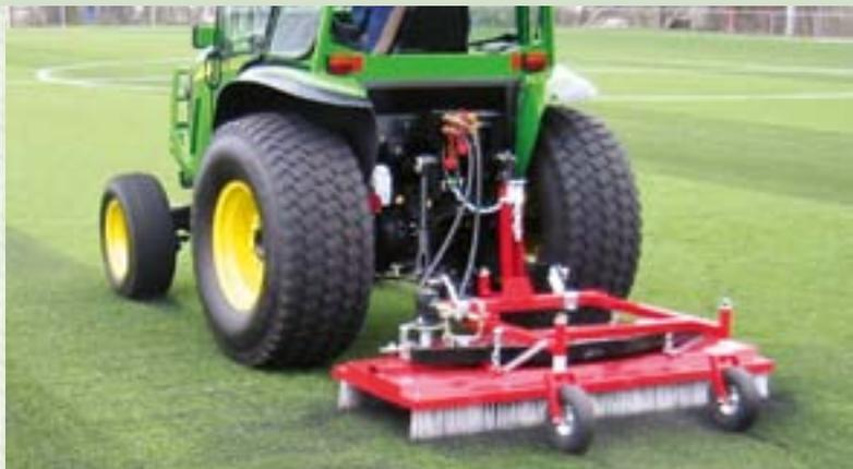
The Verti-Brush quickly and effectively levels and distributes topdressing material with powerful hydraulic brushes. The 5 counter rotating brushes can easily reach to the base of the turf to loosen and evenly redistribute fill or can be applied to mix and level a new application. The durable poly brushes can be accurately set to a specific depth to achieve a light surface brush-in or aggressively mix and loosen the deepest fill.
