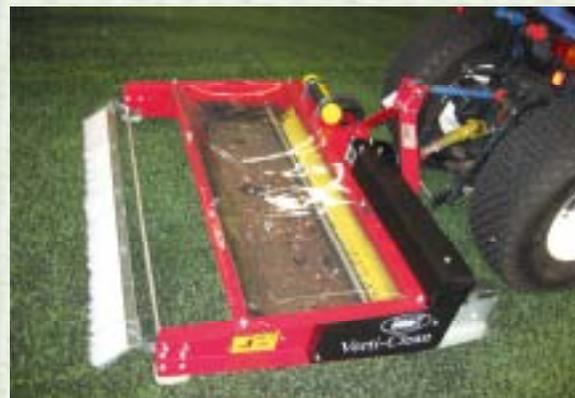
The PTO driven version of the Verti-Clean makes it easier to remove larger amounts of dirt, debris and detritus as the rotary speed of the brush can be varied.
