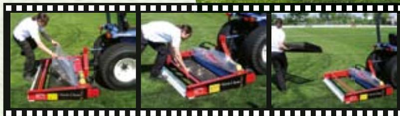
The lightweight hopper with debris can easily be removed for emptying
